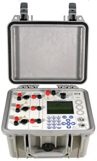
The CheckSystem 2.3 portable test system consists of an integrated three-phase current source and a three-phase electronic reference standard of accuracy class 0.2. Characteristic features of the CheckSystem 2.3 are its wide measuring range, high accuracy and high tolerance to unwanted external influences.
