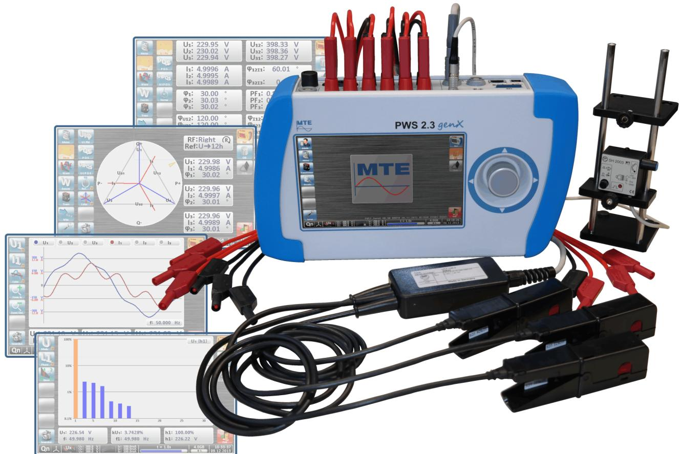
The PWS 2.3 genX Portable Working Standard is a three-phase portable electronic meter test unit of accuracy class 0.1%, used for testing single and three-phase electricity meters on site. The PWS 2.3 genX allows checking of all meter installation parameters and associated circuits.
