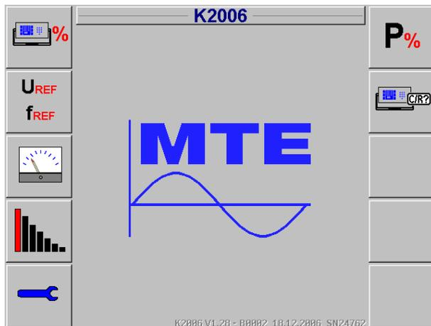
The main functions, error %, test against U-ref, f-ref, load values  $UI\phi$ , harmonics and basic system settings are directly accessed with soft keys.
