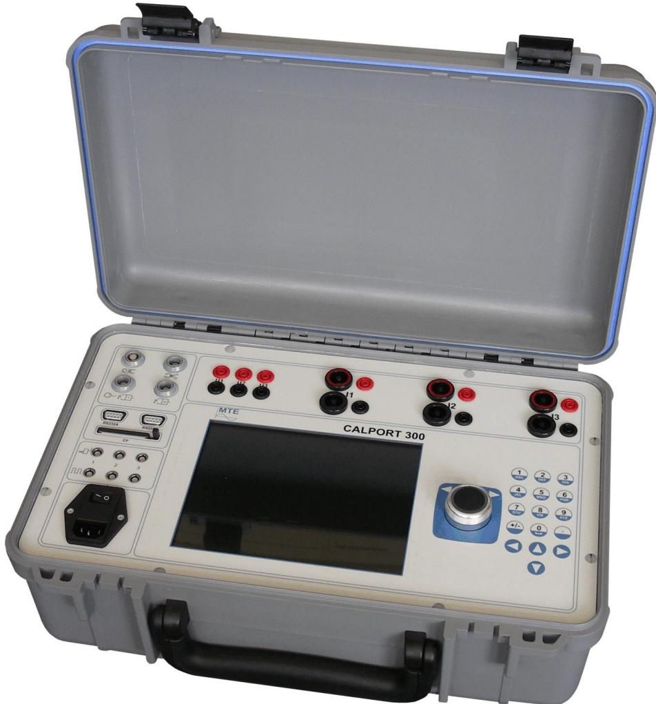
The CALPORT 300 is an universal test system for the comprehensive investigation of all components of a modern metering installation. Characteristic features are its wide measuring range, the high accuracy and the small dependence of disturbing.
