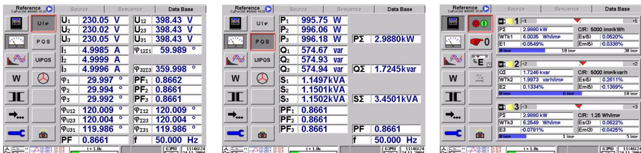
CALPORT 300 makes it possible to simultaneously test up to three electricity meters with varying constants (e.g. master and check meter of a 0.2S metering installation). Another option is a parallel test using the scanning head and the emitting contact output.
