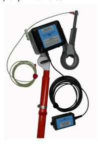
C) **590F2** is a LV, 415 to 600V primary Clip-on CT. The compensation circuit for the low voltage clamps is placed inside the 590G-V2 CT Tester.
