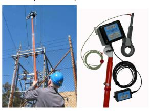
Optically isolated current clamp on the end of an insulated hotstick
